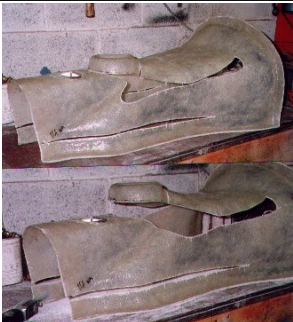
Cutting a new transmission cover to reduce the height, prior to fibre glassing.
