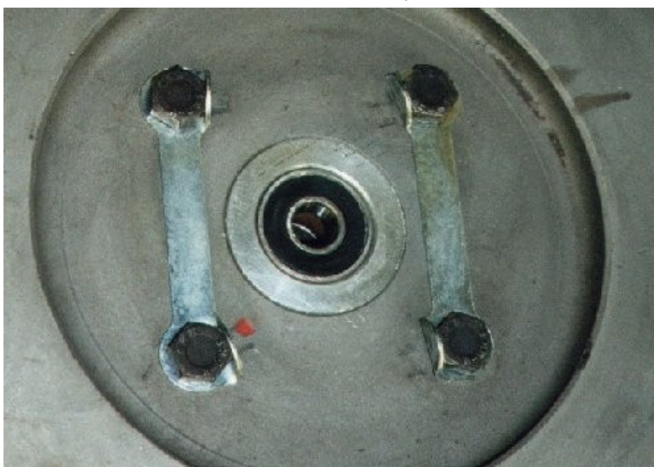
First motion shaft spigot bearing fitted to flywheel.
